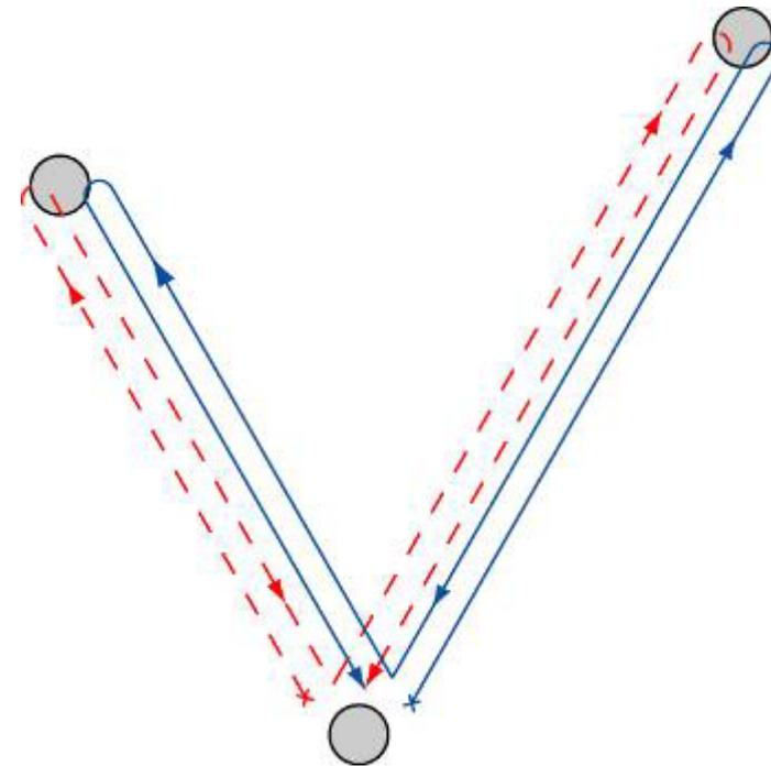
Synthesized equal-arm interferometer
